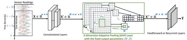
Figure 1: Overview of DAP Layer, with parameters  $(W, H)$ , that enables a DNN performing classification on input data of variable dimensions.
