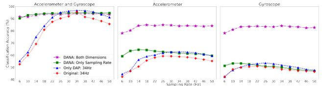
Figure 2: Classification accuracy of a benchmark DNN on UCI-HAR dataset for different sensors and sampling rate.
